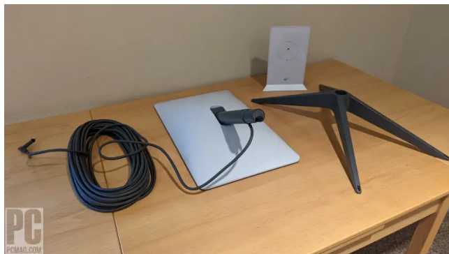
Starlink unboxing photo by Brian Westover, source: PCMag – How to Get Starlink Satellite Internet and Set It Up the Right Way [206], showing the dish, tripod and cables needed to connect to Starlink satellites.
